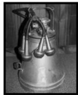
(Van, 1998). In 1892, Struthers and Weir from Scotland introduced a double chambered teat-cup. This device was claimed to produce an intermittent pressure on the teat using a rubber diaphragm to neutralize the influence of vacuum on the teat. In 1918, Carl Patrik Gustaf de Laval invented the bucket milking machine – first commercially produced and marketed machine (Roginski et al., 2003).
