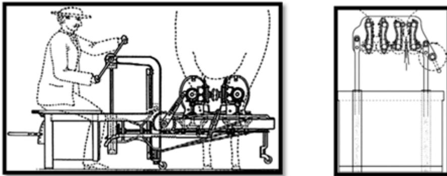
The machines were developed based on the principle of duplication of the technique of hand milking. The pressure was applied on the teat, at the attachment of the udder, closing the duct of the teat and a continuous downward pressure was applied to force the milk out of the teat cistern. Mechanically, hydraulically or pneumatically driven plates, bars, belts and rollers were used to simulate the action of hand milking (Roginski et al., 2003).
