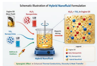
Figure 1: A schematic illustrating the formulation of a hybrid Nano fluid.
