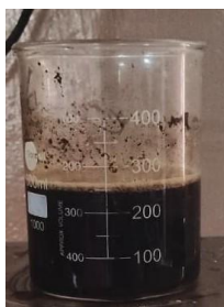
Figure 2.2(a) Extraction of Filler.
