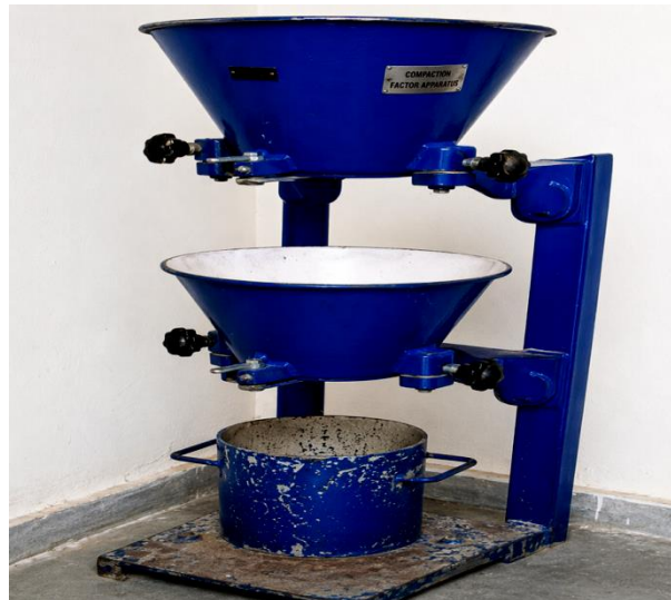
Figure 3.4 Compaction Testing Machine.
