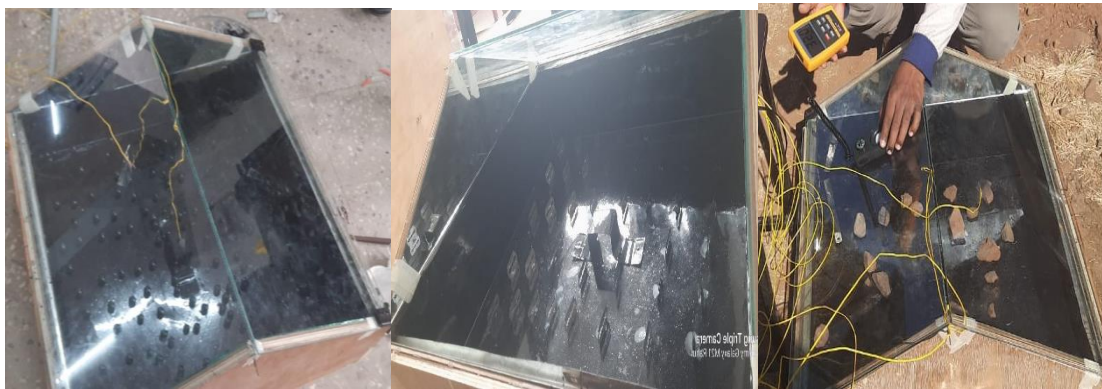
Figure 2. Arrangement of kancheys, blades and stones in solar still.
