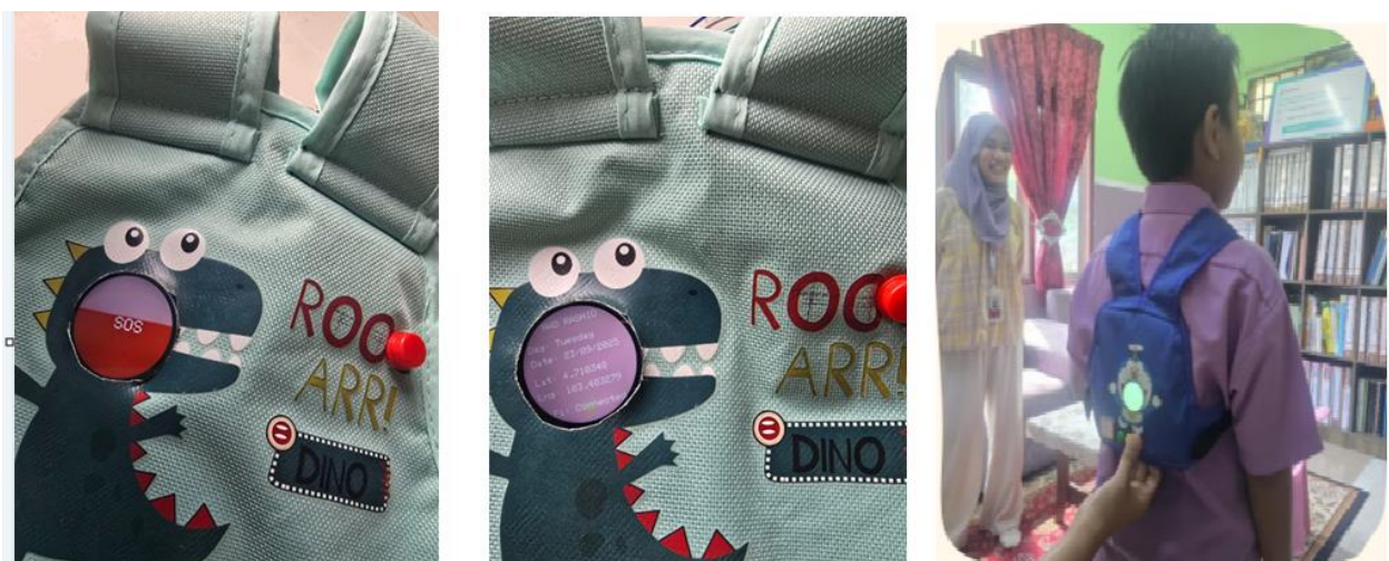
Figure 4: End product of Wearable Child Tracker with GPS and Messaging Integration.
