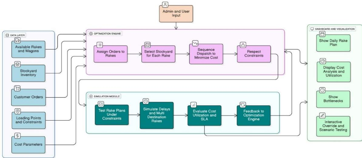
The system workflow begins with data collection from various sources, including customer orders, stockyard inventories, wagon availability, and cost parameters. These inputs are processed in the Optimization Engine, where OR-Tools algorithms assign wagons to rakes and generate cost-efficient schedules. The Simulation Module then tests these schedules under real-world constraints such as delays and multi-destination routes to evaluate performance and reliability.
