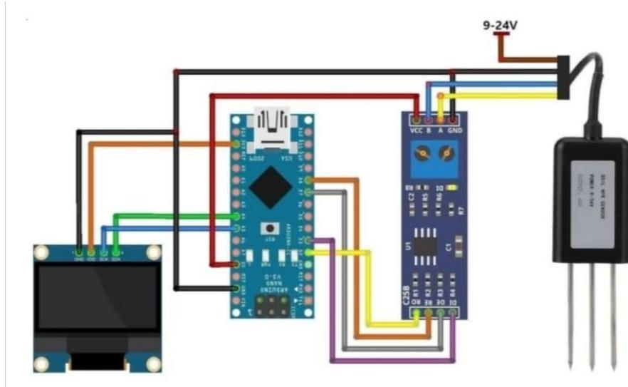
The NPK soil sensor measures the amount of Nitrogen, Phosphorus, and Potassium in the soil and sends this information as digital RS485 signals. The RS485 module converts these signals so the Arduino can read them. The Arduino receives the nutrient data, processes it, and then displays the NPK values on the OLED screen.
