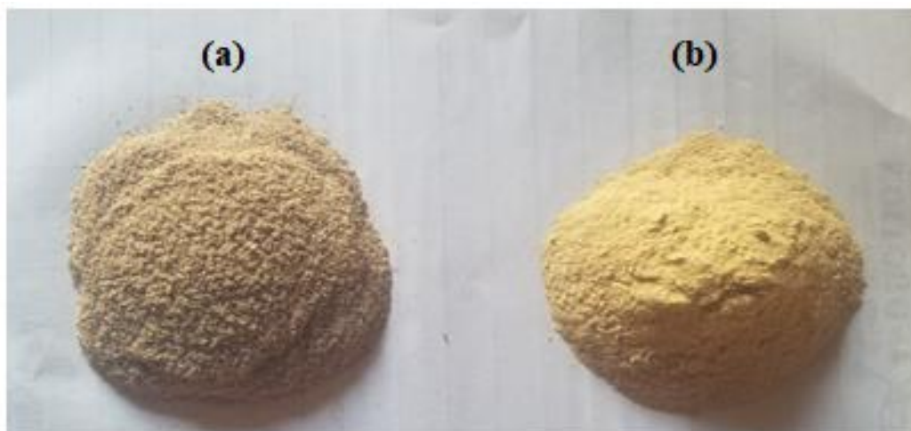
Fig. 1. Prepared and sieved raw (a) Rice husk ash (AH 1 ) and (b) Afikpo Beach sand (BH 1 )
