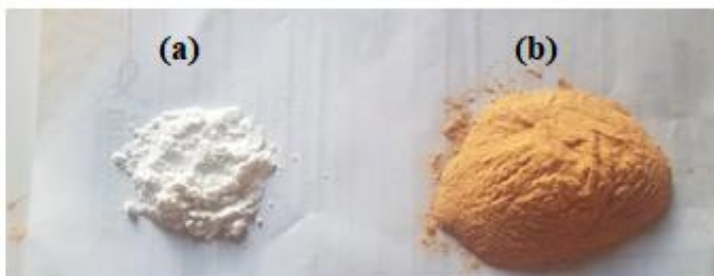
Fig. 2. Leached and calcined (a) Rice husk ash (AH 2 ) (b) Afikpo beach sand (BH 2 )
