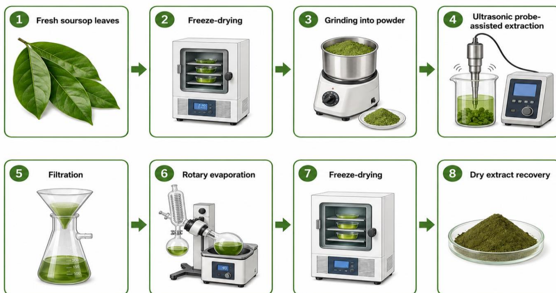
Figure 1 illustrates the extraction workflow from fresh leaves to dry extract. The sequence consisted of fresh soursop leaves, freeze-drying, powdering, ultrasonic probe-assisted extraction, filtration, rotary evaporation, freeze-drying, and recovery of the dry extract.
