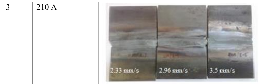
Fig. 3. Welded specimens performed with 3 different speed and current setting by conventional auto genius TIG welding process.
