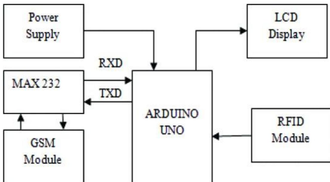
1. Power Supply provides regulated voltage to Arduino, LCD, GSM module, and RFID module to ensure proper operation.
