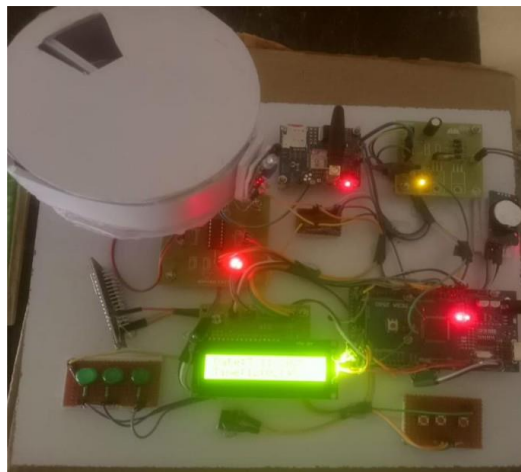
Fig. 4. Assembled hardware prototype of the IoT-based medication dispenser.
