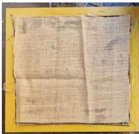
Fig. 4 Fibers arranged in the mold.
