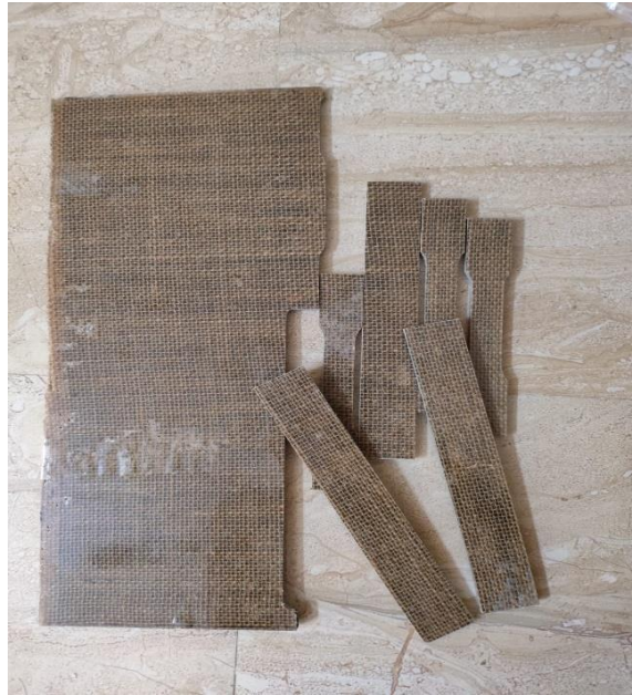
Fig.6 Specimens are cutted according to ASTM Standards.
