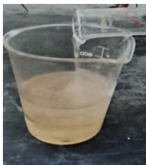
Fig. 3: Preparation of KOH–methanol catalyst solution.
