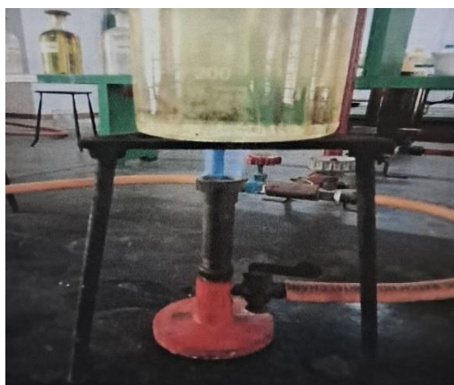
Fig. 2: Heating and conditioning of waste cooking oil prior to reaction.
