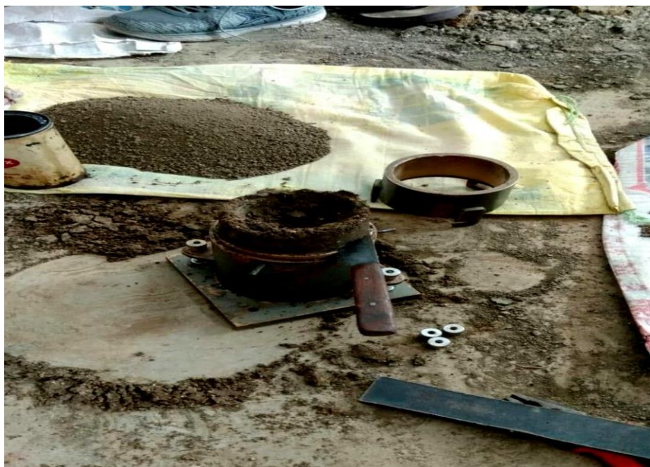
Figure 4.2 Standard Proctor Compaction Test in Laboratory.
