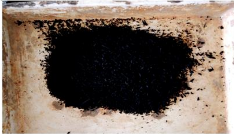
Figure 3.1 Use Crumb Rubber Tire Particles for Soil Stabilisation in an Experimental Study.
