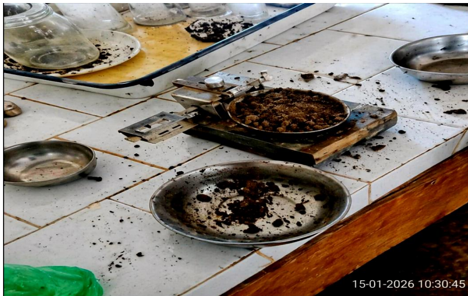
Figure 4.1 Experimental Setup for Liquid Limit Determination Using Casagrande Apparatus
