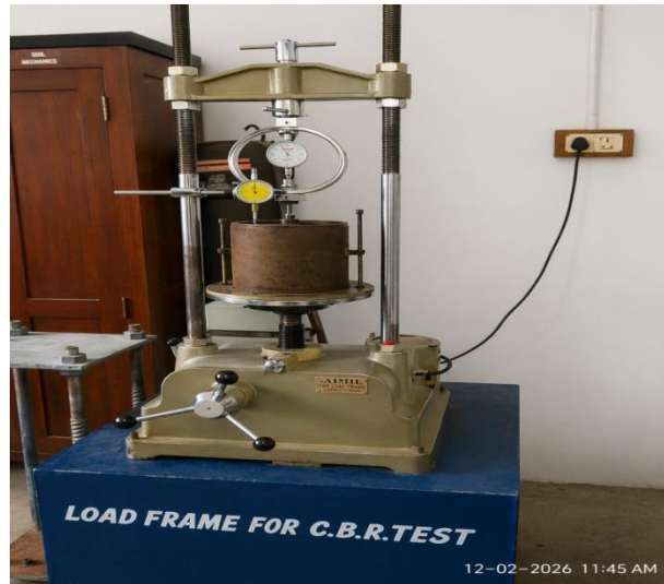
Figure 4.4 Load Frame Setup for California Bearing Ratio (CBR) Test.
